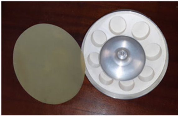
Fig. 7. Fabrication of the final inverted-hat antenna.
