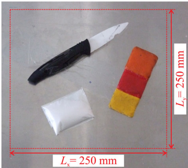
Fig. 4. Scene of dielectric threat objects, consisting of a kitchen knife with ceramic blade, a stepped bee wax sheet with different thicknesses d_1 = 5.0 mm (yellow part), d_2 = 10.0 mm (red part), and d_3 = 15.0 mm (orange part) with relative permittivity \epsilon_r \approx 2.3 and a small bag filled with table salt (NaCl). All objects are attached to a metal plate. The red dashed line indicates the fully polarimetric imaged area for both mono- and multistatic measurement setups.
