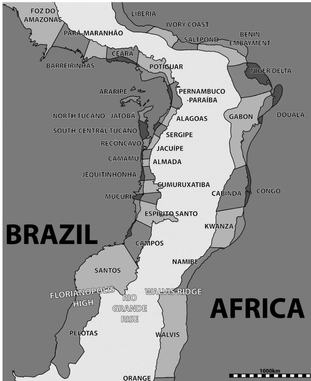
FIGURE 1—Schematic map of the offshore basins surrounding the South Atlantic Ocean, demonstrating the close conjugation of the coastlines of eastern Brazil and western Africa. The oceanward extents of the basins are represented by the 3,000 m bathymetric depth line, which approximately corresponds to the ocean-continent boundary. The positions of three structural features (Florianópolis High, Rio Grande Rise, and Walvis Ridge) which together prevented the influx of oceanic water into the proto-South Atlantic from further south are indicated. Adapted from Coward et al. (1999), with Brazilian basin names and extents modified following the work of Milani et al. (2007).
