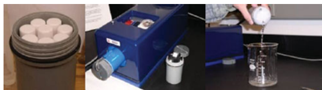
Figure 2. (Color online) McCrone micronizing mill and its accessories.
