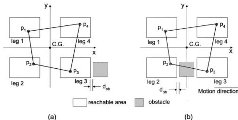
Fig. 4. Influence of obstacle on the gait: (a) the obstacle is of DIO type for Leg 3 and of SIO for Leg 2, (b) the obstacle is of DIO type for Leg 2 and of SIO for Leg 4.
