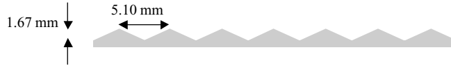
FIGURE 2. Profile of the upper and lower boundaries. The pitch at the inner wall is 4.9 mm, and at the outer wall is 5.3 mm. The depth of the teeth is 1.42 mm at the inner wall and 1.92 mm at the outside. The figure shows the average pitch and depth of the teeth.
