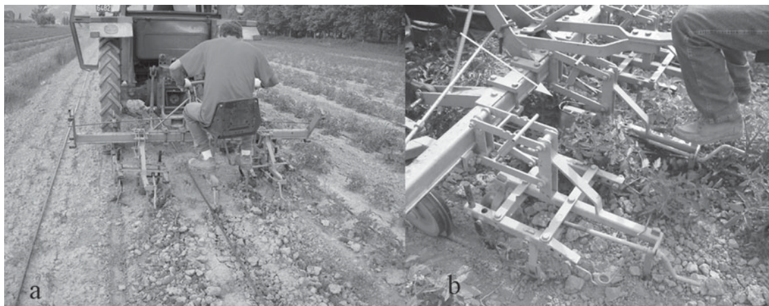
Figure 5. (a) Early precision hoeing treatment performed, with a machine designed and developed at the University of Pisa, in processing tomato without removing the drip line between paired rows in 2007; (b) late precision hoeing in 2006. The hoe was equipped with ‘V’-shaped elements in order to open the developed crop vegetation.
