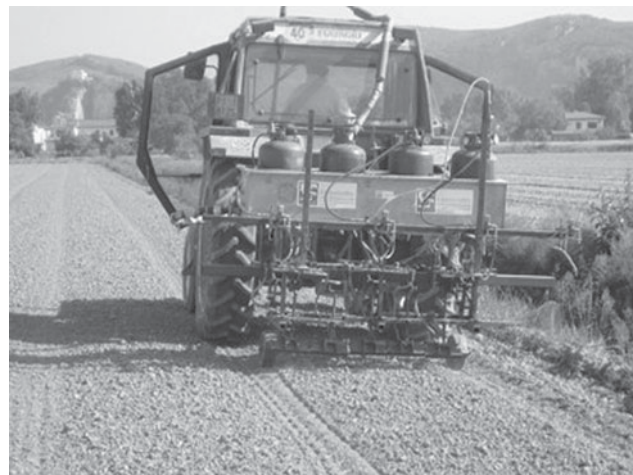
Figure 4. Flaming machine, designed and developed at the University of Pisa, in a field near Pisa, Italy, in 2008 during a pre-transplanting weed control treatment on processing tomato.
