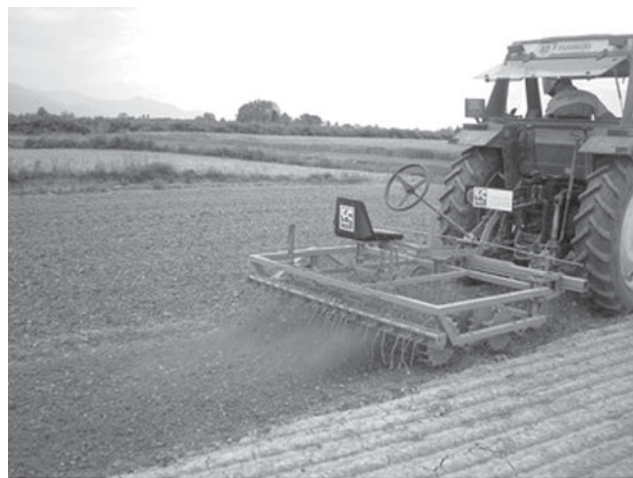
Figure 3. Rolling harrow, designed and developed at the University of Pisa, equipped with flexible teeth and used during a pre-transplanting weed control treatment on processing tomato near Pisa, Italy, in 2008.
