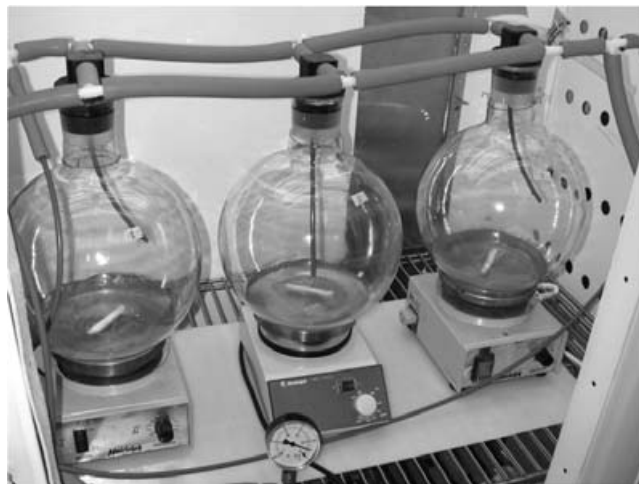
Fig. 1. Underpressurized culture vials, used for Synechocystis cell cultivations, were located in a growth chamber. The CO 2 -enriched, water-saturated air was led down into the bottles through plastic tubes. The liquid cultures were gently stirred (120 rpm) using magnetic stirrers under the bottles. A gauge controlled the vacuum.
