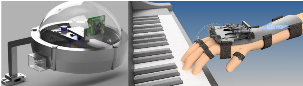
Figure 3: Camera system for the handbike to safely assess the traffic situation and orthosis for the drop hand
