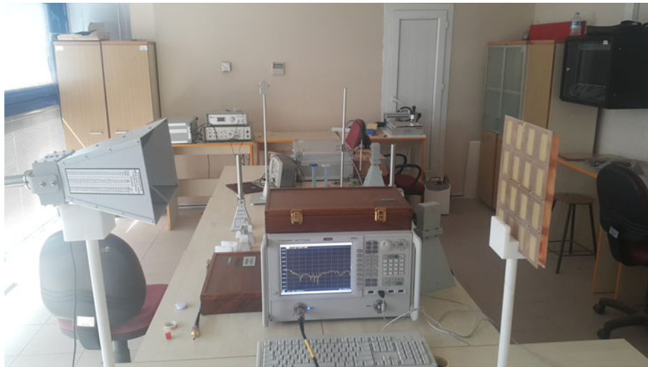
Fig. 3. Laboratory test picture using single-horn antennas, a 42.5 GHz Agilent vector network analyzer.
