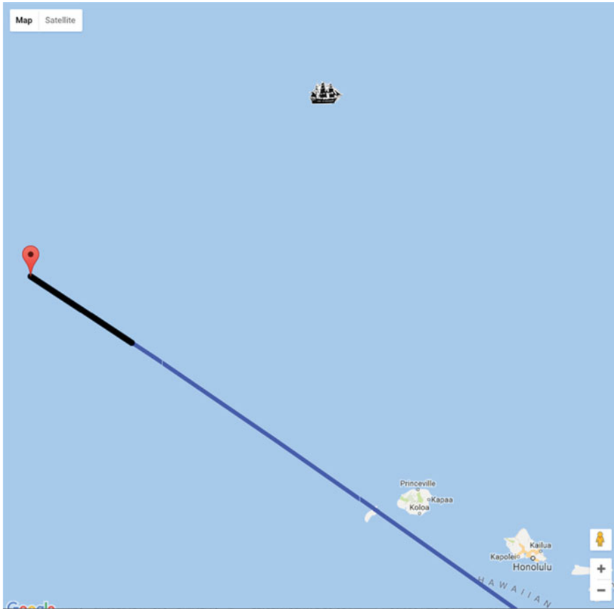
Figure 5. The intercept line drawn as the thick black line leading toward the GP, relative to the AP.
