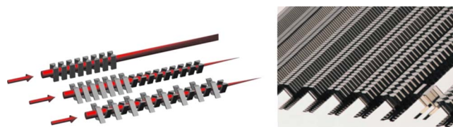
Figure 6. (Color online) Left: refractive X-ray lenses, arranged in series and alternating. Right: SU-8 polymer lenses on a Si wafer.
