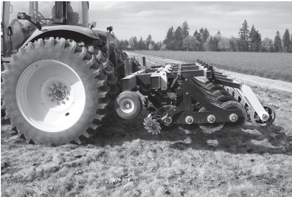
Figure 2. A second-pass strip tillage machine was developed by Hendricks Farms (Stayton, OR) and modified by Pearmine Farmers (Gervais, OR). Multiple gangs of parallel disks and a sprocket roller break up soil clods to prepare a seed bed within the tilled crop zones.
