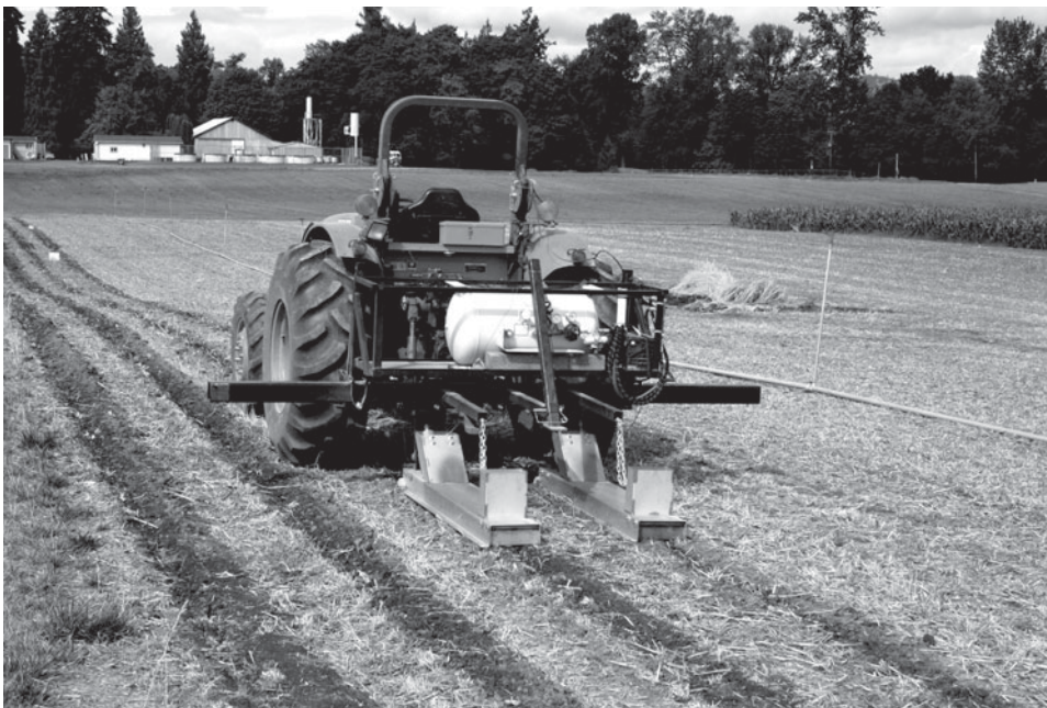
Figure 3. A strip flamer, developed by Charles Merfield and modified by Edward Peachey at Oregon State University, can be used in organic zone tillage systems to reduce weeds in the crop row.
