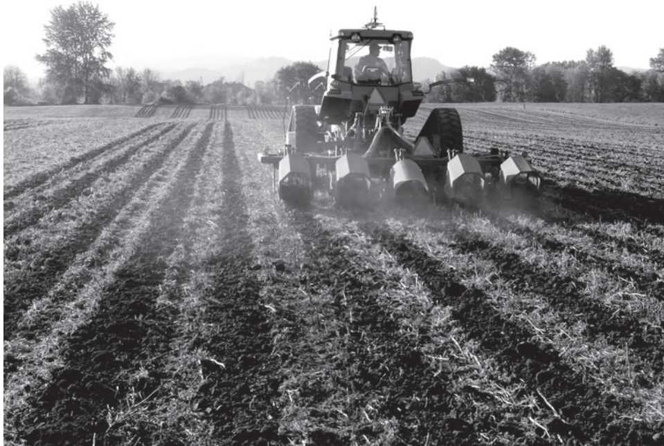
Figure 1. Zone tillage involves separate tillage, weed control and fertilizer operations for the crop zone and the between-row zones. The shank/coulter strip tillage machine shown here tills strips approximately 25 cm wide and 30 cm deep.
