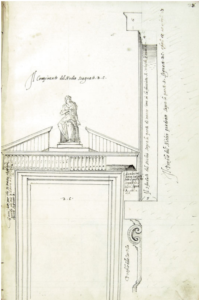
Fig. 16. Galeazzo Alessi, frame marked B.C. with its pediment for the exterior façade of S. Maria presso S. Celso (Milan, Biblioteca Ambrosiana, S. 149 Sup. B, fol. 8; with permission)
