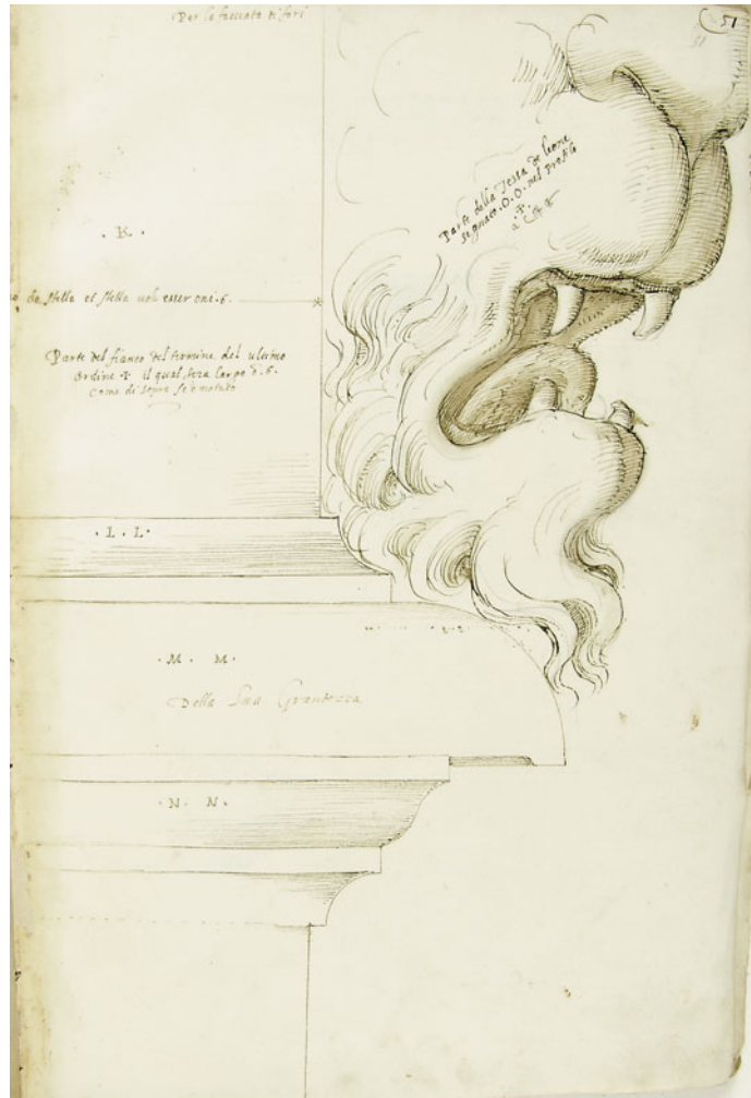
Fig. 17. Galeazzo Alessi, life-size drawing of the moulding of the leonine order for the exterior façade of S. Maria presso S. Celso (Milan, Biblioteca Ambrosiana, S. 149 Sup. B, fol. 51; with permission)
