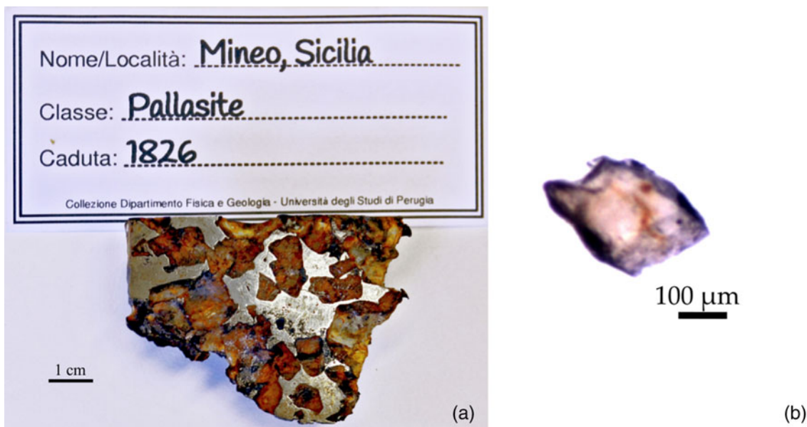
Fig. 1. (a) Photo of the Mineo pallasite portion owned by the Department of Physics and Geology of the University of Perugia (sample no. Mineo1969.SL3P#002 CNR inventory 213248); (b) isolated olivine single crystal from the Mineo pallasite where a reddish area is observed.
