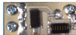
Fig. 5. Schematic (left) and photograph (right) of a 2 nd order low-pass filter with 700 MHz cut-off for the proposed ET system in Fig. 4 to suppress all harmonics higher than modulation bandwidth; C1 = 7.5 pF, C2 = 5.2 pF, L1 = 18 nH, L2 = 16 nH.
