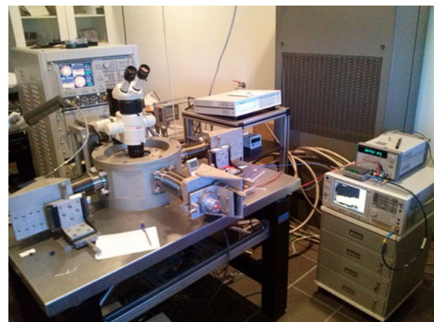
Fig. 6. Picture of the custom cryogenic probe station.
