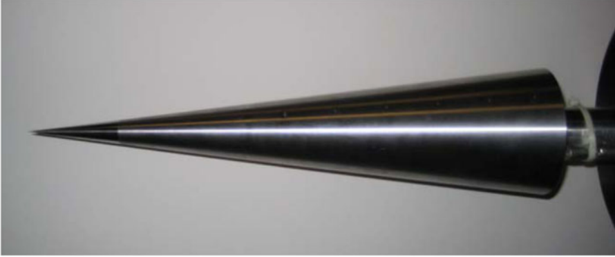
FIGURE 1. Cone model used in the Purdue experiments (S. P. Schneider 2009, private communication).
