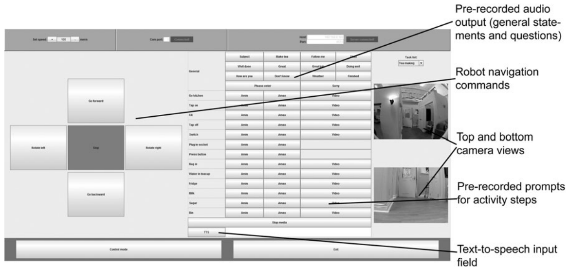
Figure 2. Display of tele-operator's screen, indicating commands available to the operator during the study.
