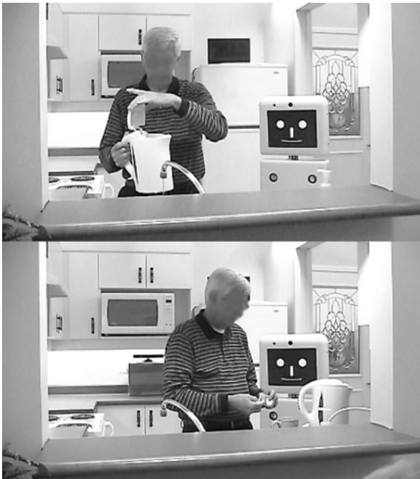
Figure 3. Tele-operated assistive robot, “Ed”, assisting a participant to make a cup of tea in the kitchen.
