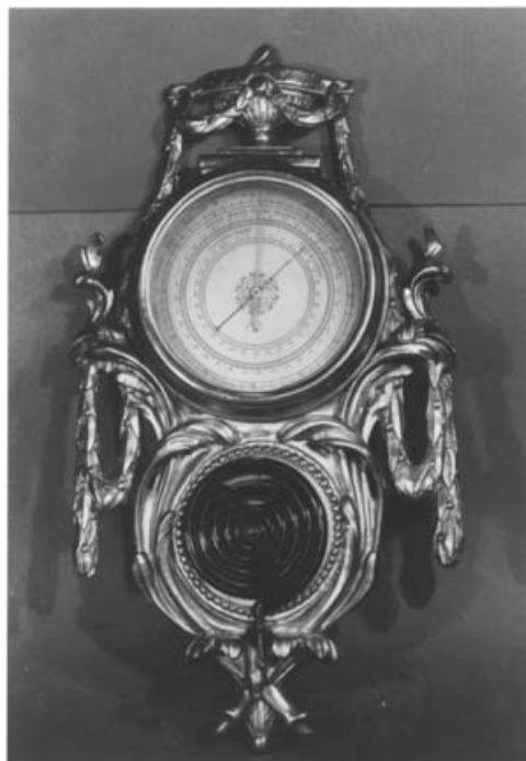
Figure 1. Spiral thermometer ‘after Fahrenheit’s scale’, made by Bianchy & Comp. à Amsterdam (Musée des Arts & Métier-CNAM, Paris/Photo Studio CNAM).
