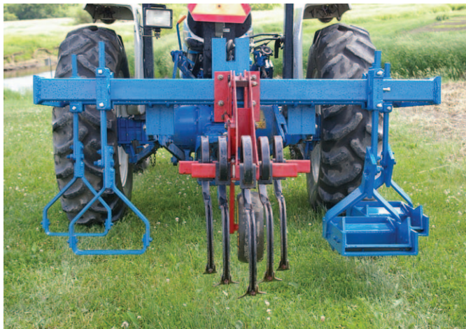
Figure 1. Rear view of the toolbar and the three different cultivator designs. Left to right: stirrup, sweep, and block cultivators.
