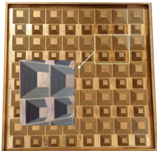
Fig. 4. Experimental realization of two layer hybrid ultra-broadband absorber for absorption from S to Ka band. This figure is reproduced with permission from [69]. © 2015, Nature Publishing Group.
