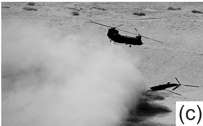
Figure 7. Geometry of the brownout cloud that is produced by a tandem-rotor helicopter when operating close to the ground: (a) hover mode, (b) recirculatory mode, (c) ground vortex mode. (all individual images Crown copyright)
