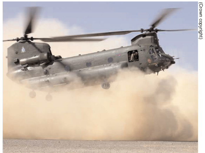
Figure 1. Chinook helicopter landing in dusty conditions. Note the cloud of dust that is being produced below the aircraft; brownout is a distinct possibility should the aircraft decelerate or descend.
