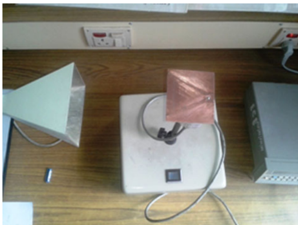
Fig. 9. Testing of radiation pattern of horn antenna on X-band microwave test bench.
