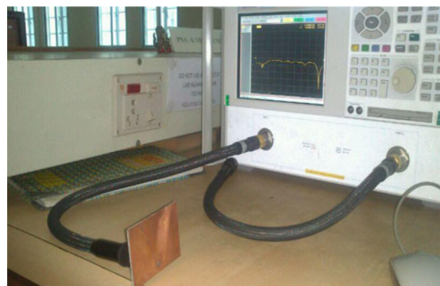
Fig. 6. S-parameter measurement of horn antenna using VNA.
