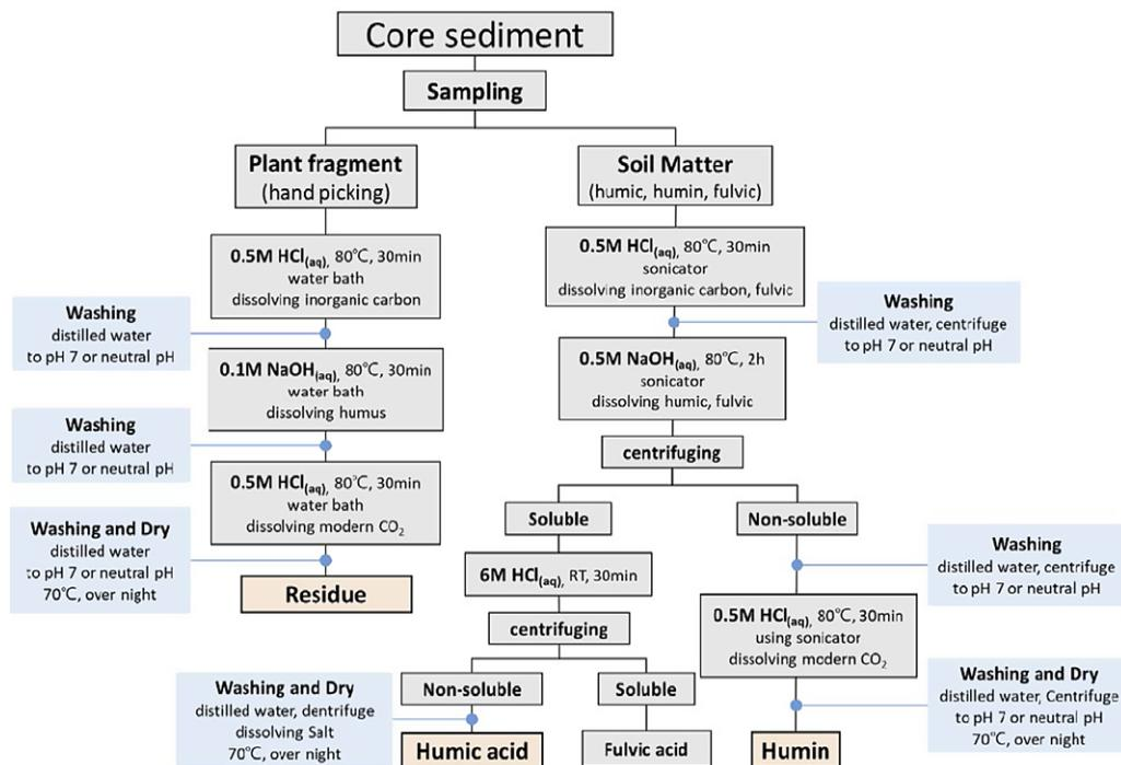
Figure 2 Schematic diagram of the pretreatment procedure for  $^{14}\text{C}$  dating materials (modified from Kigoshi et al. 1980; Kretschmer et al. 1997).
