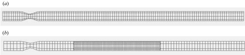
FIGURE 2. Layout of spectral element mesh. (a) Axisymmetric stenosis model with K = 2240 hexahedral cells, and (b) eccentric stenosis model with K = 2448 hexahedral cells.
