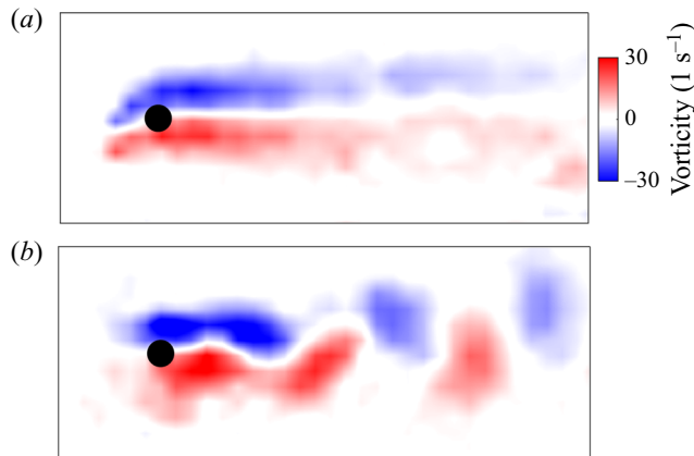
Figure 2. The wake of a fixed cylinder at (a) Re = 33 and (b) Re = 60 .
