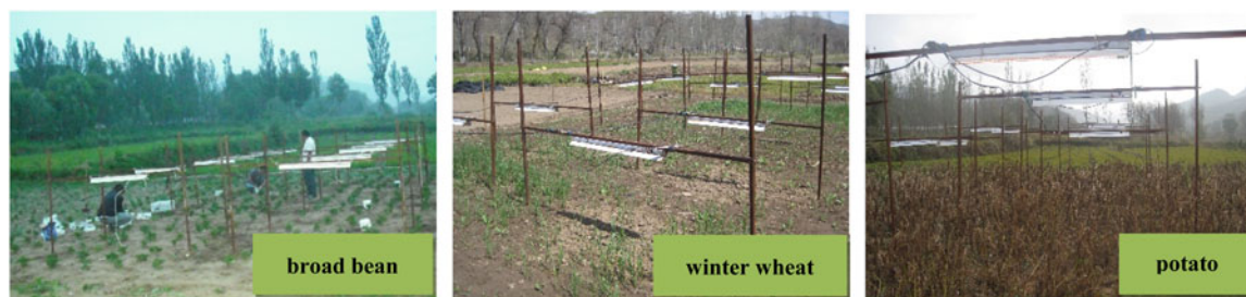
Fig. 1. (Colour online) A farm heating system using infrared ray radiators during the growing season of the potato–broad bean–winter wheat rotation system at Guyuan Agricultural Meteorology Experiment Station in a semi-arid area of China.
