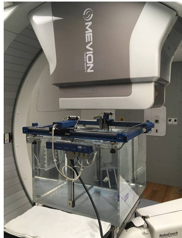
Figure 2. IDs measurement with IBA Blue phantom setup.
