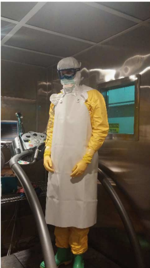
Subject Outfitted to Start a Test Wearing the E3 Personal Protective Equipment Ensemble.
