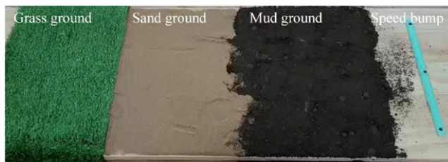
Figure 14. Connecting the grass ground, sand ground, mud ground, and speed bump to construct a mixed complex ground.
