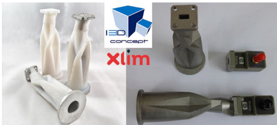
Fig. 11. Manufactured mode converter made out of plastic (left) and stainless steel (right) before measurement.
