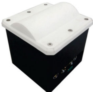
Fig. 8. Prototype setup of the presented radar system with the dielectric lens. Overall dimensions 75 mm × 75 mm × 60 mm
