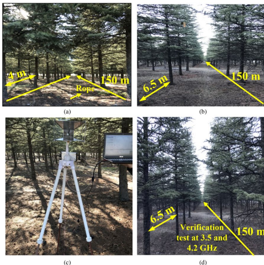
Fig. 7. Reference and verification measurement environments for 3.5 and 4.2 GHz.
