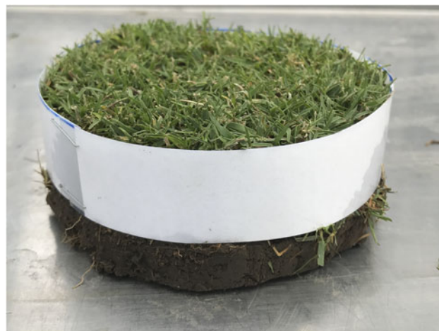
Figure 1. A plastic band was used to prevent leaf area from expanding beyond the original core size and to prevent spray deposition on the leading edge of the core so the core would receive spray as it would in situ.
