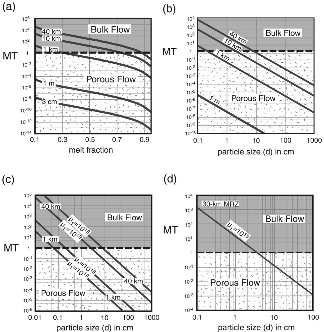
**Figure 3** The results of the melt transport (MT) number calculations. For the values of the parameters used, see Table 1. (a) Effect of pluton/melt-rich zone (MRZ) size (e.g. 40 km) on MT number at particle size of 3 mm and  $\mu_1=10^{18}$  poise. (b) Effect of MRZ/particle size on MT number at 0.4 melt fraction. (c) Effect of viscosity and MRZ size on MT number at 0.4 melt fraction. (d) Melt transport number calculation for the LM as a 30 km MRZ at 0.5 melt fraction (see text).
