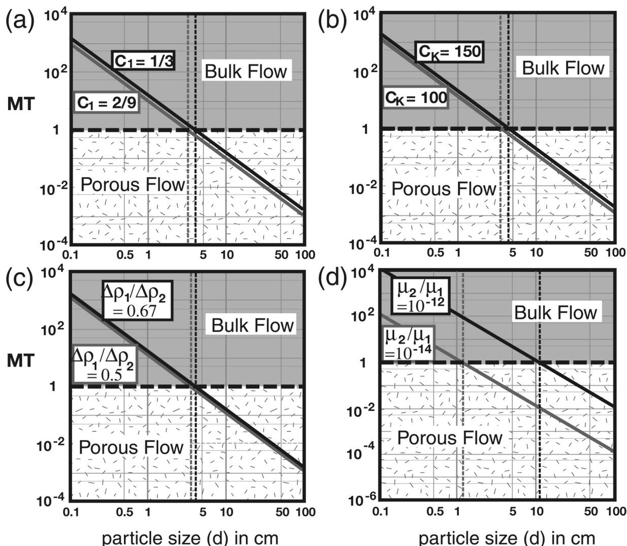
**Figure 4** Further results of the melt transport (MT) number calculations showing the effects of varied values for the parameters on MT number at 0.5 melt fraction for a 30 km melt-rich zone: effects of: (a) viscosity constant; (b) permeability constant; (c) density difference; and (d) viscosity difference. For the values of the other parameters used, see Table 1.
