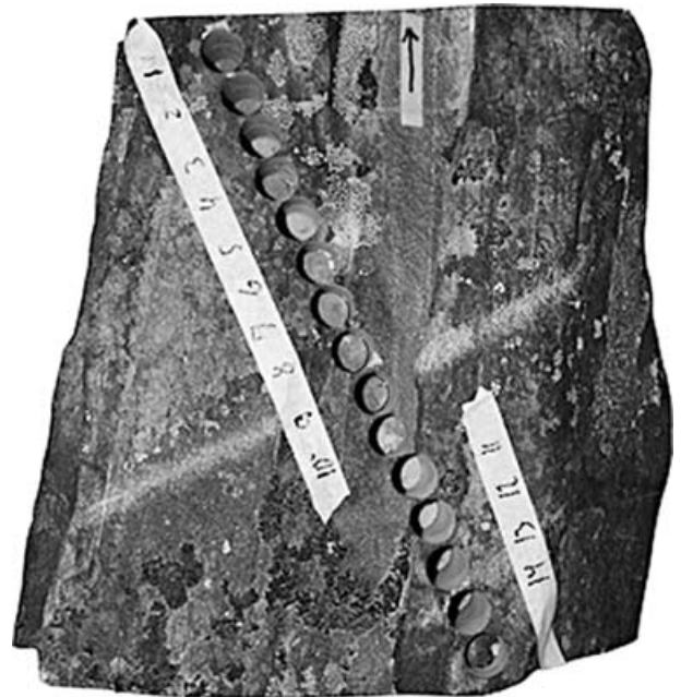
Figure 2. Amphibolite boulder with trace of the first lightning. Fourteen samples have been drilled out of the boulder along a line perpendicular to the EW-oriented trace of the lightning. The figures on the tape indicate sampling sites along an NS-oriented profile. Sample 1 is the northernmost sample. Length of drilling profile is about 40 cm.
