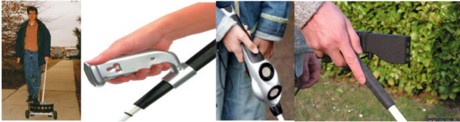
Figure 1. From left: Robotised smart cane, smart cane (K-Sonar), intelligent canes (UltraCane, TomPouce).
