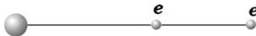
Fig. 6. Sketch of the classical frozen planet configuration (Richter and Wintgen 1990), which is a stable configuration of the unperturbed, classical three body Coulomb dynamics. Both electrons are located on the same side of the nucleus. In the collinear configuration shown, the outer electron is standing still at a fixed point in space, while the inner electron performs rapid oscillations along an extremal parabolic orbit of eccentricity one. The configuration is the result of a dynamical stabilisation phenomenon, which emerges from the competition of the various Coulomb interaction terms in the helium Hamiltonian.
