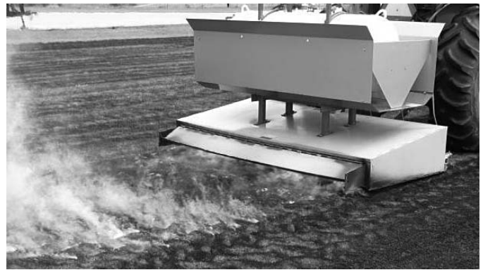
Figure 1. PL8750 flame sanitizer demonstrating short thermal heat exposure by flame.
