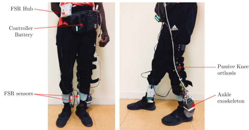
Fig. 8. A parietic patient wearing the ankle joint exoskeleton and the FSR sensors.
