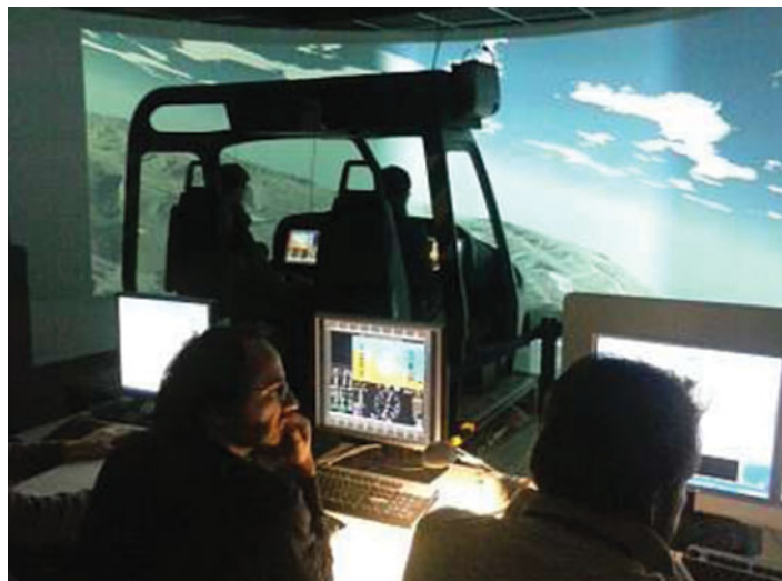
Figure 4. Image from the AW169 tail rotor loss simulation trials (Leonardo) (11).
