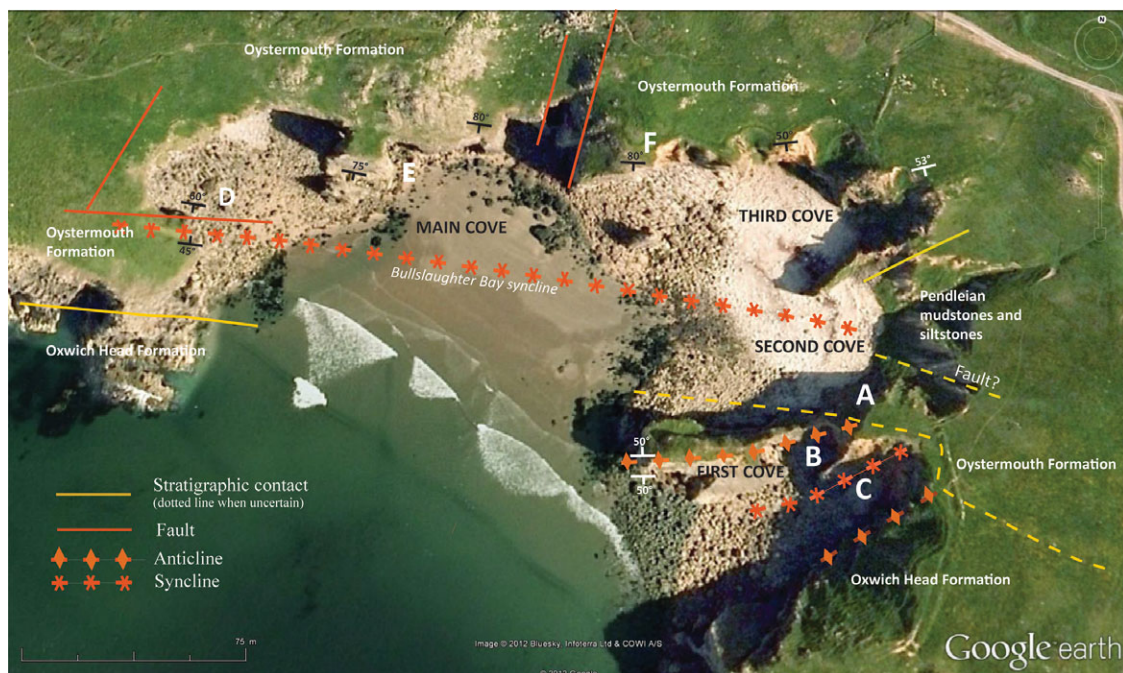
Fig. 4. (Colour online) Geological sketch of Bullslaughter Bay showing the main significant structures. The Oxwich Head Formation crops out on the west side of the bay south of the Bullslaughter Bay Syncline, and also on the southeast side. 'Gash-Breccias' are not indicated. A, B, C, D, E and F mark the sampling sites. (Sources: Dixon, 1921; Thomas, 1971; background from Google Earth © 2012 Bluesky, Infoterra Ltd & COWI A/S.)
