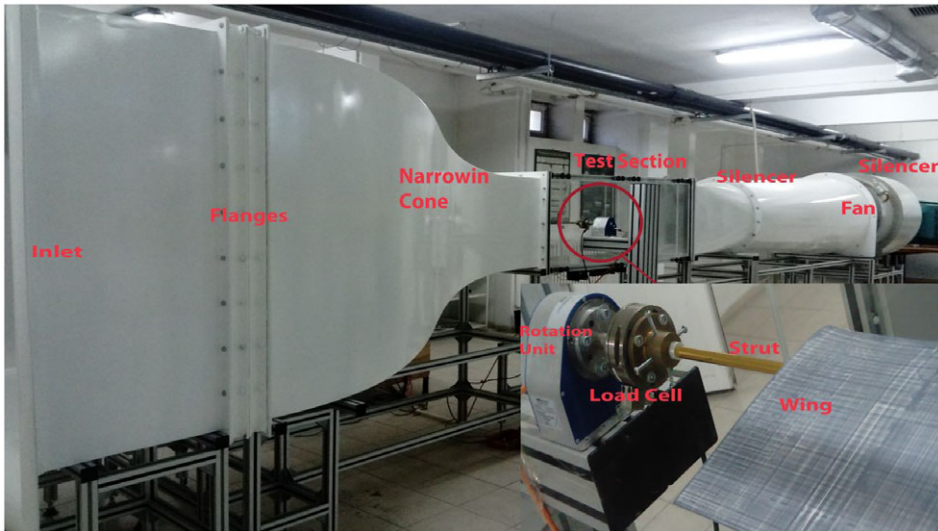
Figure 2. Wind tunnel and detailed view of the test section.
