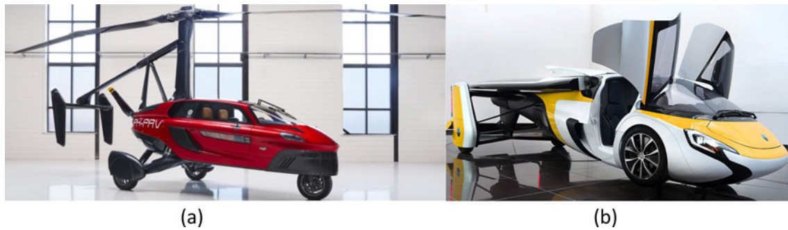
Fig. 3. Examples of flying cars: (a) VTOL designed by PAL-V 4 and (b) STOL designed by Aeromobil 5 .
