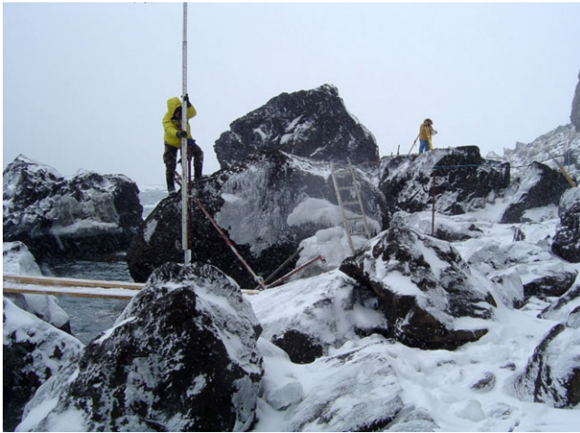
Fig. 16. Surveyors record position of a temporary tide gauge. Courtesy NIWA. Reference W2pKsHvR.
