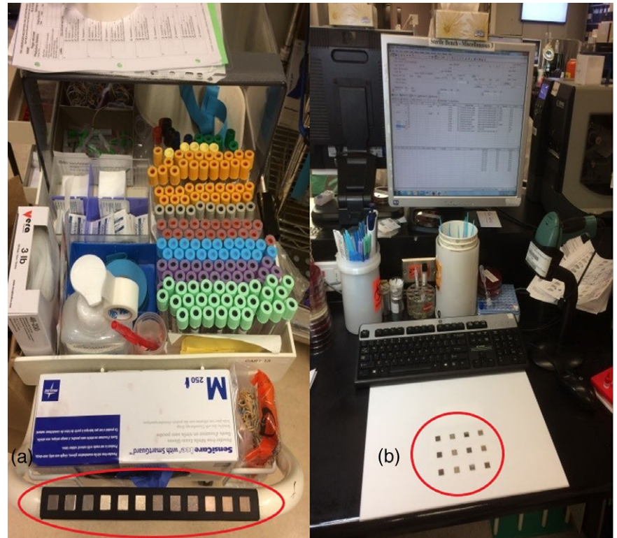
Fig 1. Examples of (A) cart gasket affixed to a phlebotomy cart handle on a clinical unit and (B) medical microbiology laboratory bench gasket. All gaskets contained stainless-steel and copper-formulation coupons (1 cm 2 ) in triplicate (red circles).
