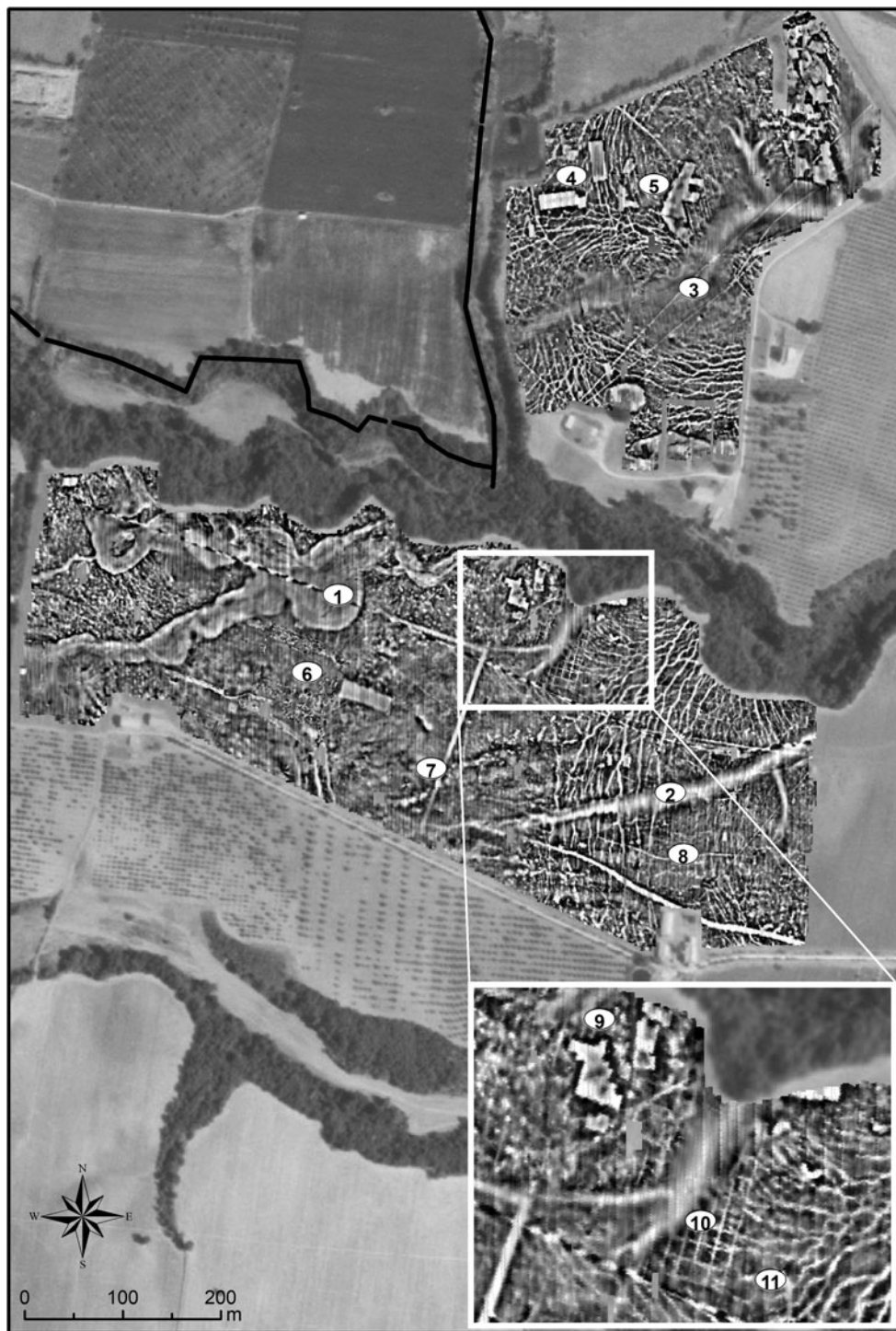
Fig. 2. – Results of the magnetometry survey in the eastern and southern fields. Data range -100 nt (white) +100 nt (black). Numbers follow the order of described features in the text.
