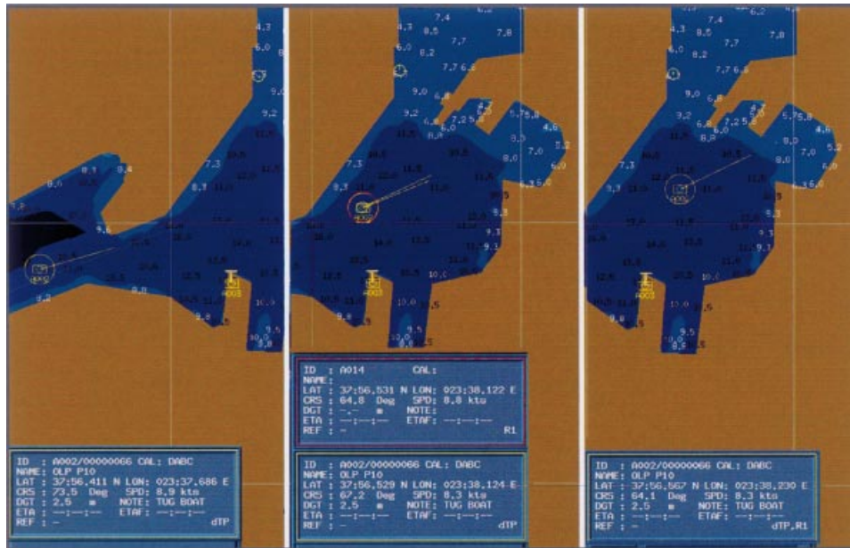
Figure 5. Track fusion: left – AIS track; middle – separate radar and AIS tracks; right – track fusion of radar and AIS.
