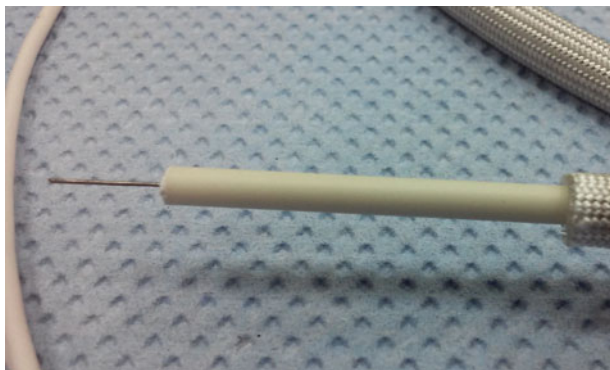
Fig. 7. Langmuir probe manufactured in the PlANS laboratory.
